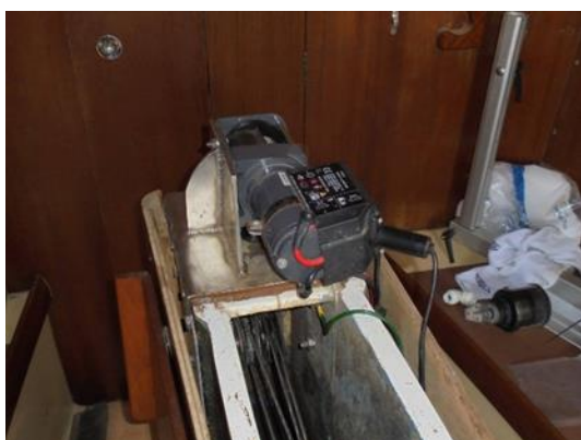
Mechanized keel lifting mechanism; a truck's winch.
