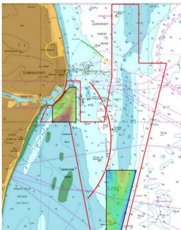
Approaches to Lowestoft. The highlighted areas indicate where bathymetric surveys are carried out twice yearly. The mud banks shift position every season.
