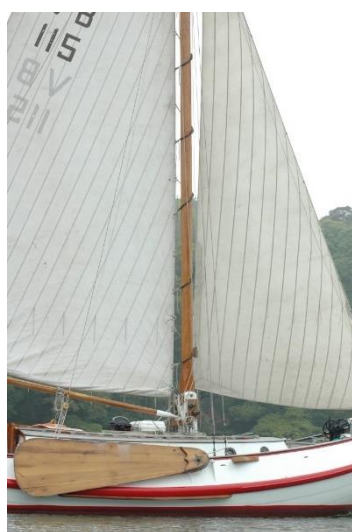
Sail lashing technique in a Dutch sailing barge.
