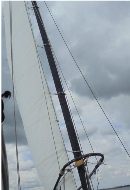
Nausikaa's sails attached with bead parrels.
