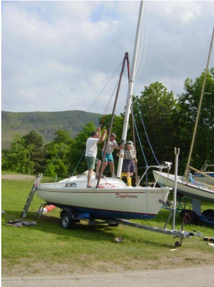
Photo 5: Here the mast has cleared the coach roof and is about to be positioned above the mast hole. Notice how little effort is now needed from the helpers to position the mast.
