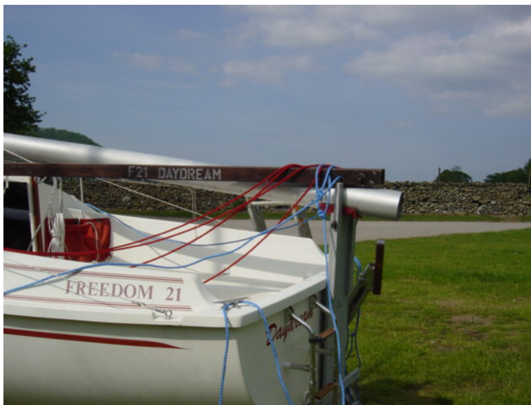
Photo 2: The top of the bi-pod sheer legs rests on the foot of the mast ready for hoisting – the blue lines are the fore and aft supporting guys. It is sufficient to just tie-off the guys to the top of the sheer legs with bowlines – the loads involved are really low.
