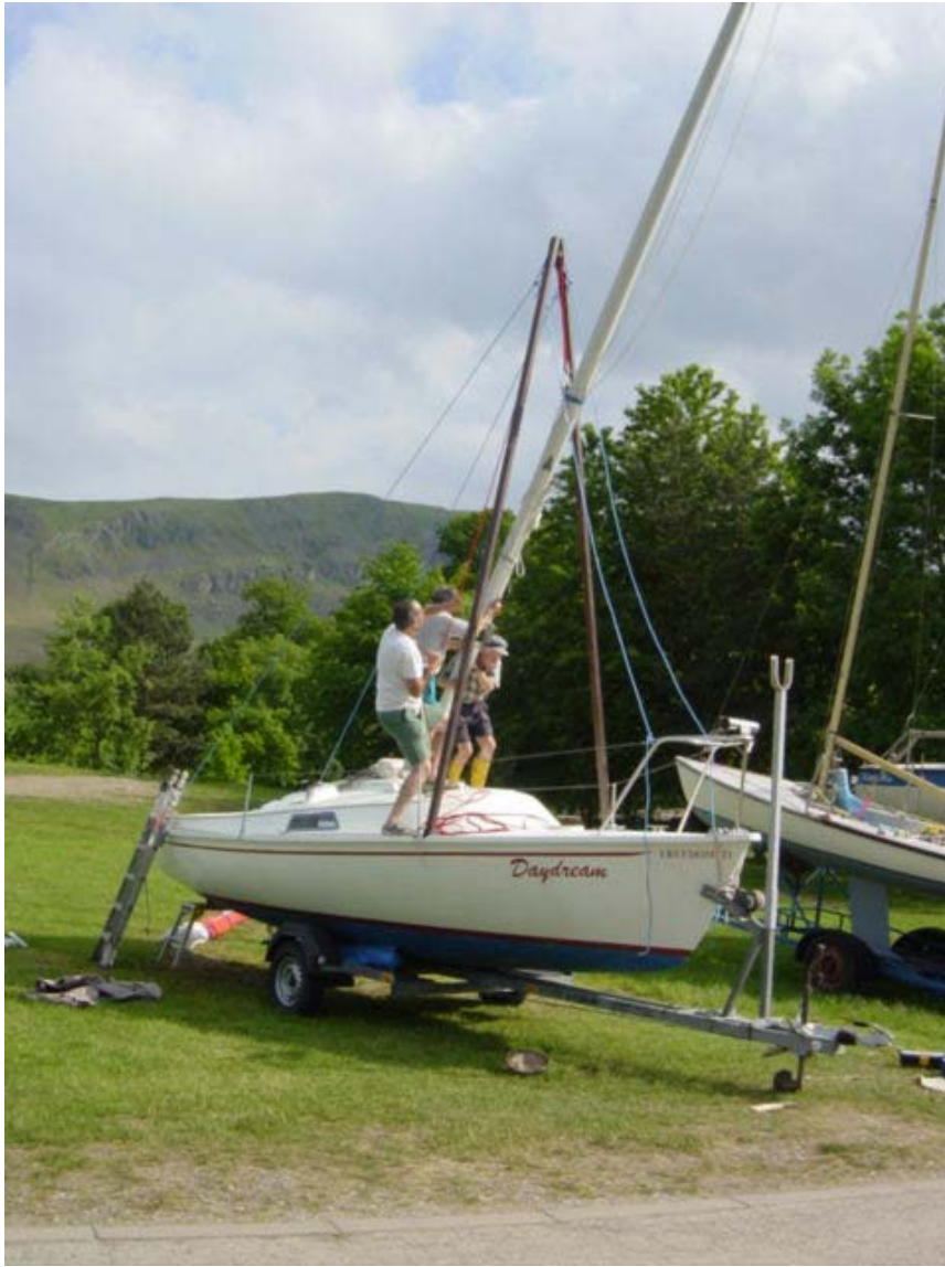
Photo 4: This is the start of the mast lifting operation. I am on the starboard side of the boat hoisting on the lifting tackle whilst two helpers are guiding the mast as it pivots into a vertical position. It is important to hoist the mast sufficiently high enough to allow the mast foot to clear the coach roof as it pivots into the vertical. All of the mast weight is taken by the lifting tackle but it is essential to have helpers controlling the mast as otherwise it would be free to swing about with rather impressive ease – especially in anything of a breeze!
