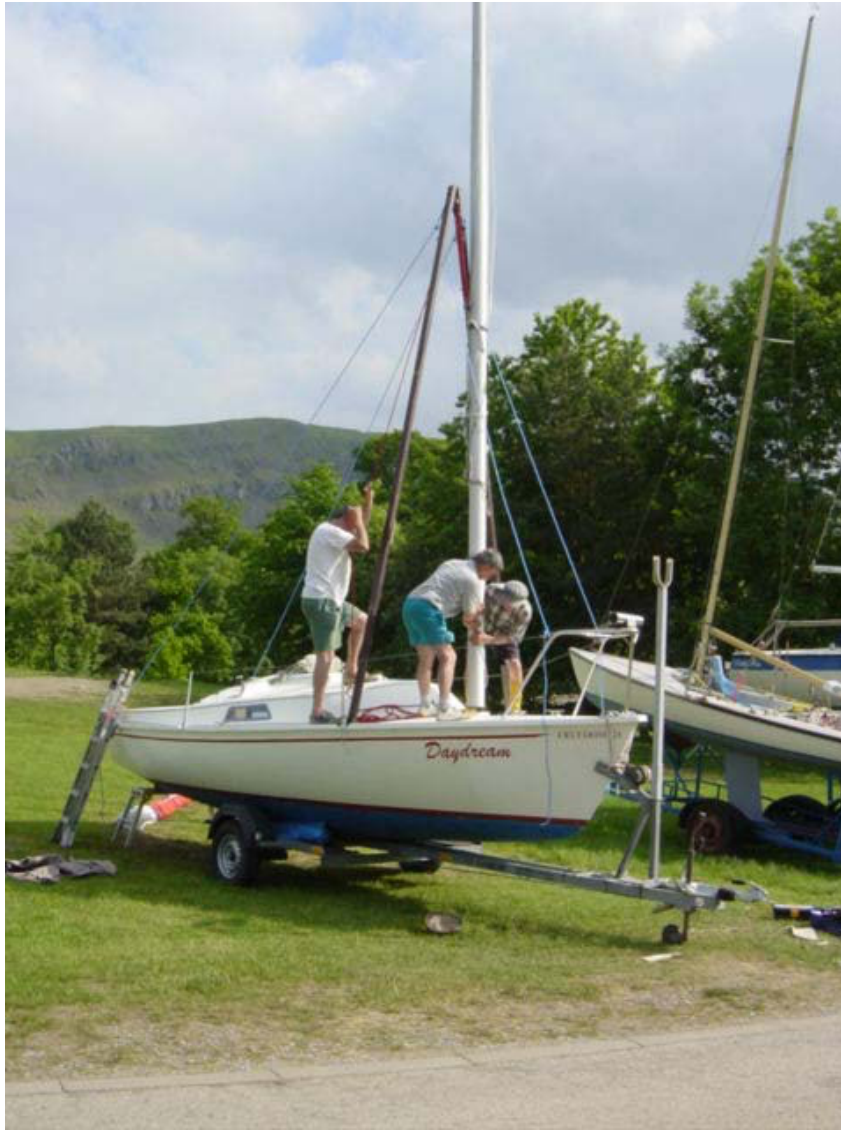
Photo 6: Finally in goes the mast – I can then hand over the hoisting tackle, go below and align the mast foot as it comes down on the male spigot on the keel. Again – take great care to keep fingers well clear of the mast foot as it drops down onto the spigot, as it is certainly a dangerous item on heavy UK masts but still a broken finger potential on the lightweight USA carbon fibre masts?
