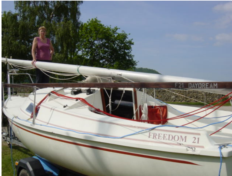
Photo 1: The bi-pod sheer legs are shown here laid out – resting on the wire guard rails and the mast foot with all rigging & lines attached ready for mast hoisting. It looks a bit of jumble but if all lines are attached & neatly laid-out this helps the operation run smoothly.
