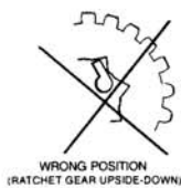
VIEW OF RATCHET GEAR PAWLS
